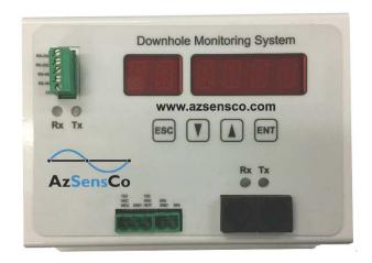
The ASR100 is the readout unit for the APS400 Series transducer. The readout provides both temperature and pressure for the APS400.
