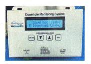
Press the DOWN Arrow key to save the changes or the UP Arrow key to discard the changes. The menu will return to the Overview Menu and will cycle through the readings.
