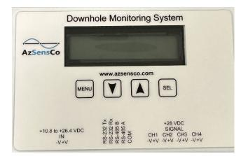
The ASR240I is the surface readout unit for the APS400/APS420 series transducers. It has a built-in optical isolation filter per IPC-2221.
