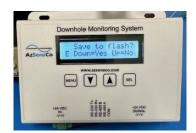
Press Select Button to step through menu Items. See menu tables below for SRU models. To change a parameter, press the up or down arrow keys. To save the change, press the menu button.
